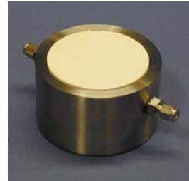
Fig. 3 HAEPD bonded into a standard triaxial pedestal
