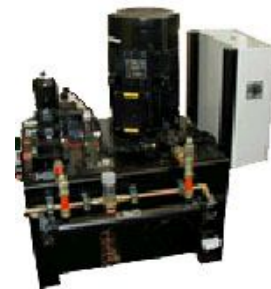
Fig. 2 GDS 25MPa hydraulic power unit
