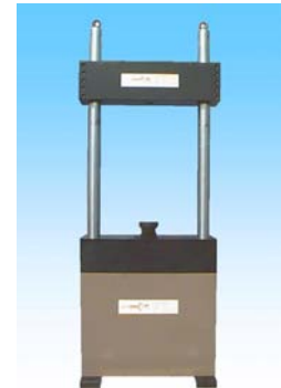
GDS axial loading Frame, range from 10kN to 500kN
