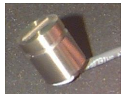
Fig. 1 GDS Titanium Bender Element and Insert
