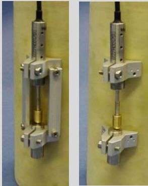
Fig 1: Axial local strain transducers mounted directly on a triaxial test specimen
