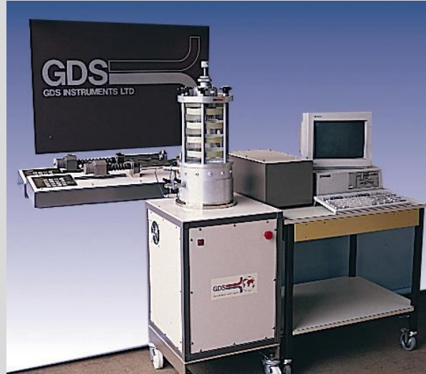
2Hz, 40kN, 2MPa DYNTTS system shown above
