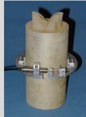
Fig 2: Radial local strain transducers mounted directly on a triaxial test specimen
